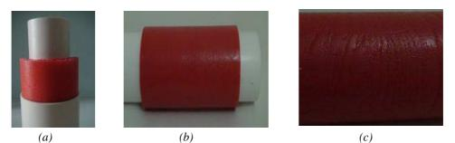
Figure 3: Sample obtained with use of teflon and solid vaseline applied to the inner wall of the PVC pipe.
