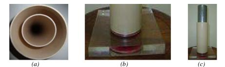
Figure 2: Positioning of concentric tubes (a) and the acrylic base (b) and (c) to formation of mold.
