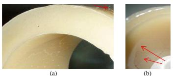
Figure 6:. Sample obtained using two PVC pipes, Carnaud wax and PVA liquid as a release agent applied to the inner and outer walls of the inner tube and the inner wall of the outer tube.
