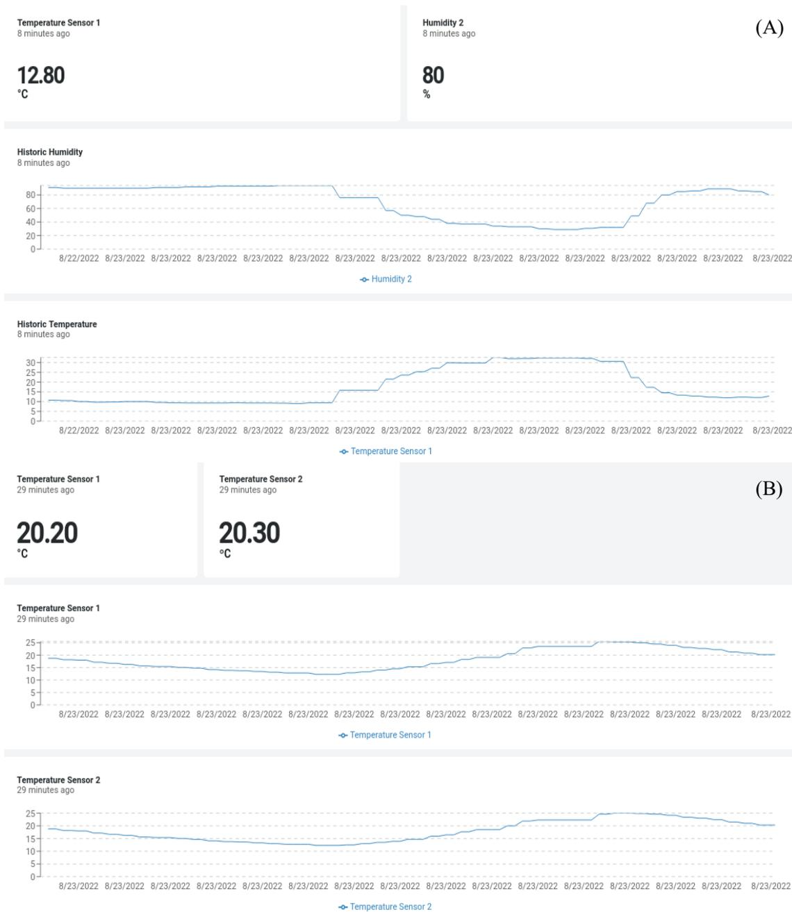
Figure 4: Dashboard with Datacake integration representing the air temperature and relative humidity sensor (A) and the substrate temperature of one end-device (B).
