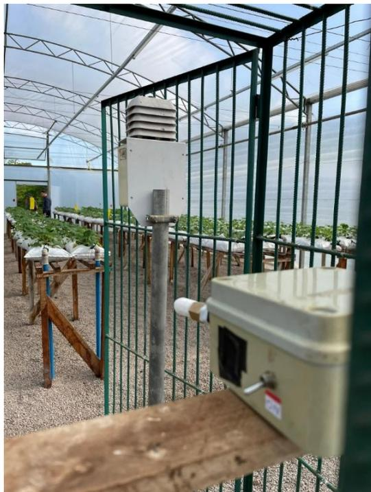
*Figure 3: Device equipped with the SHT20 sensor to measure air temperature and relative humidity.*
