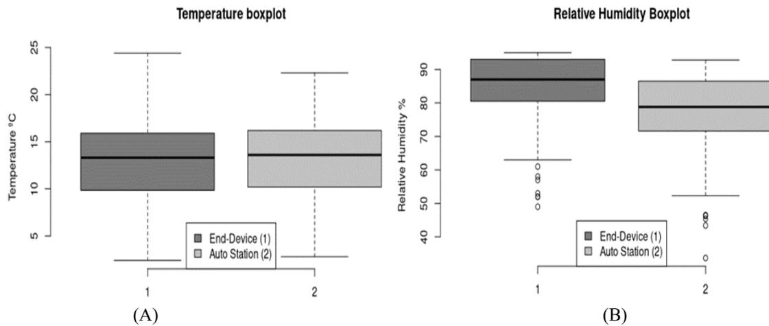
Figure 5: Air temperature (A) and relative humidity (B) from the SHT20 sensor (1) and automatic station (2).
