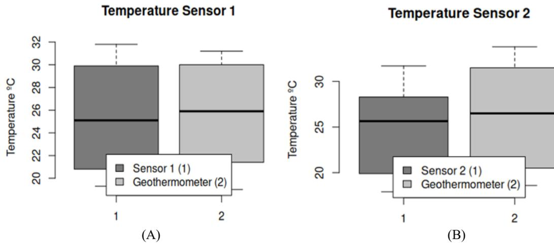
Figure 6: Comparison of Substrate Temperature between Sensor and Geothermometer 1 (A) and Sensor and Geothermometer 2 (B).
