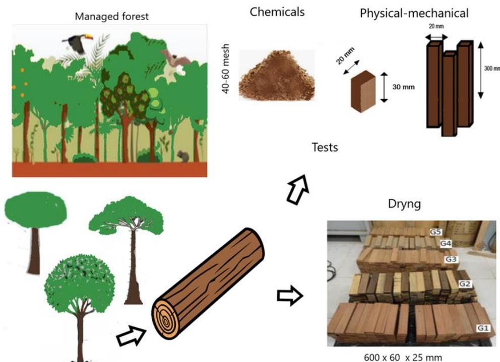
Figure 1. Scheme of the sampling and preparation of specimens.
