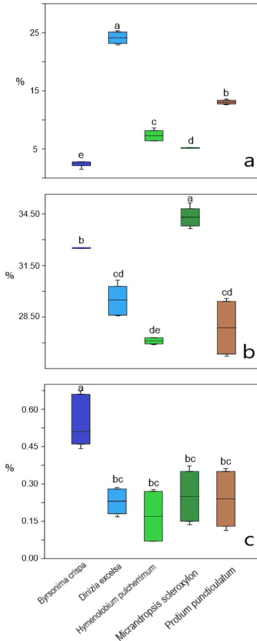
Figure 3. Results of the chemical properties of the studied woods: a – Extractives; b – Lignin; c – Ash. Bar = standard error  $\pm 1\%$  represents the 99% confidence interval. Groups designated by identical letters within the column exhibit no statistically significant differences according to Tukey's test at the 5% probability level.
