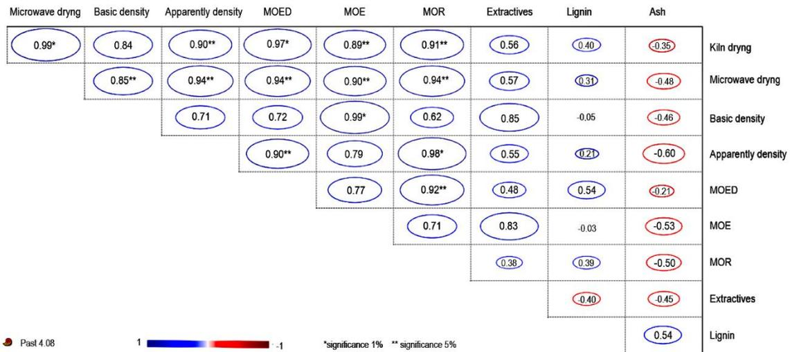
Figure 4: Result of Pearson's analysis based on the correlation between the chemical and physical-mechanical properties of the wood studied. MOED = Dynamic modulus of elasticity; MOE = Modulus of elasticity and MOR = Modulus of rupture in static bending.
