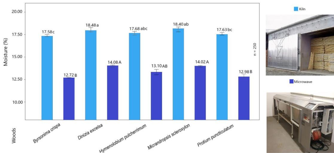
Figure 2. Results of moisture in the woods studied. Bar = standard error  $\pm 1\%$  represents the 99% confidence interval. Groups designated by identical letters within the column exhibit no statistically significant differences according to Tukey's test at the 5% probability level.
