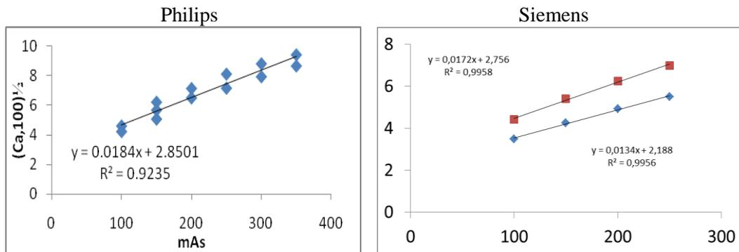
Figure 7: CT air kerma index ( $C_{a,100}$ ) vs. mAs for both scanners.
