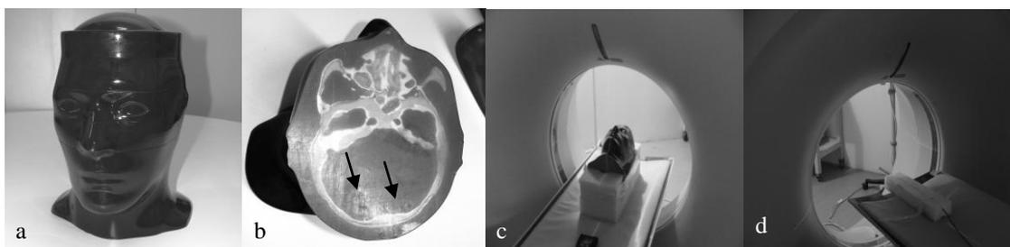
Figure 1: a) RS-250 Head head phantom; b) posterior fossa phantom section, pointing to the lesions; c) phantom positioned in the CT scanner; d) air kerma in air measurement with a pencil ionization chamber.
