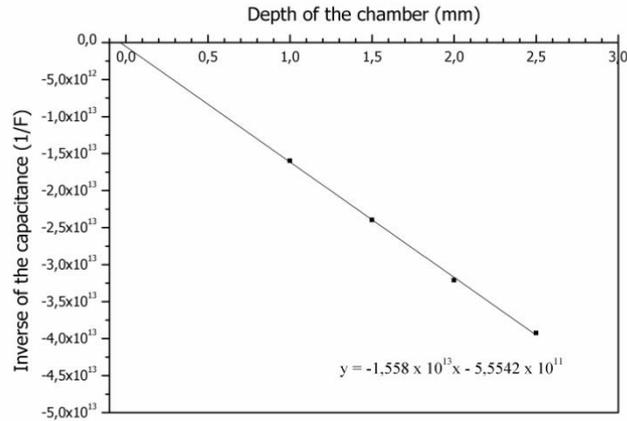
Figura 3: Extrapolation line of the 23392 PTW chamber in  $^{90}\text{Sr}/^{90}\text{Y}$  beta radiation beam.
